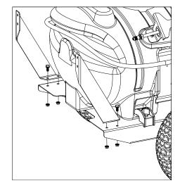
Attach the boom mounts to the frame. Make sure the brackets are parallel with each other before tightening down the bolts.
